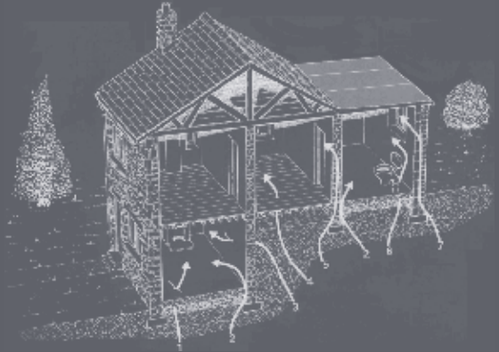
Figure 1 Routes by which radon enters a dwelling
